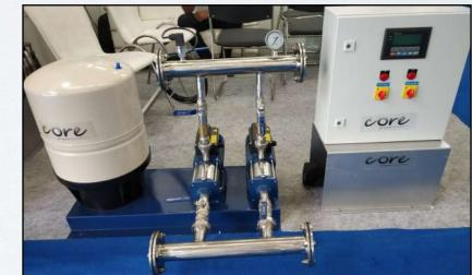
Any centrifugal pump driven by a constant/variable speed electric motor. The number of stages in these feed pumps is determined by the feed quantity and discharge pressure. Sometimes a combination of number of pumps with an air operated system is also used, which is known as hydro-pneumatic pumping systems
